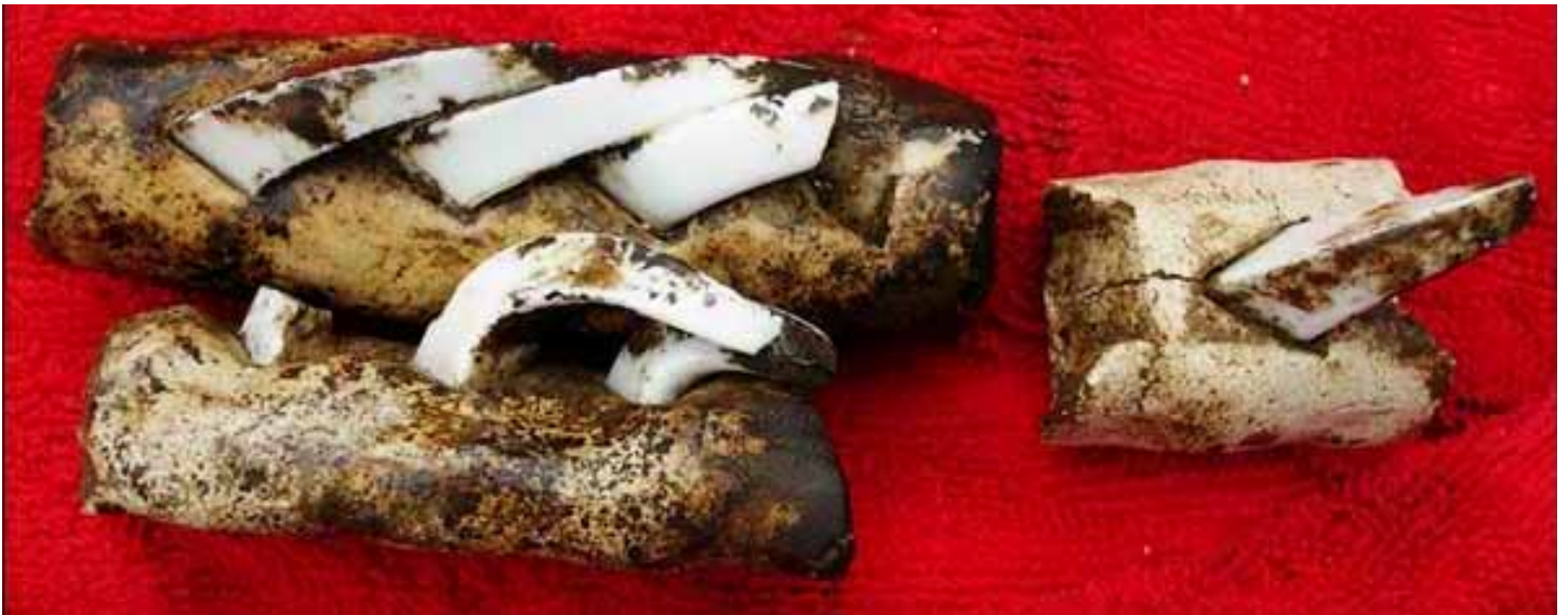
Above: A series of three cones were used when firing the ware to the correct temperature. One would be the guide cone, the middle one the firing cone and the third the guard cone. Each slumps as it reaches a different temperature. Below: A pottery cone, Rho Dendra shards and what is believed to be chunks of Rho Dendra-colored pink clay.
