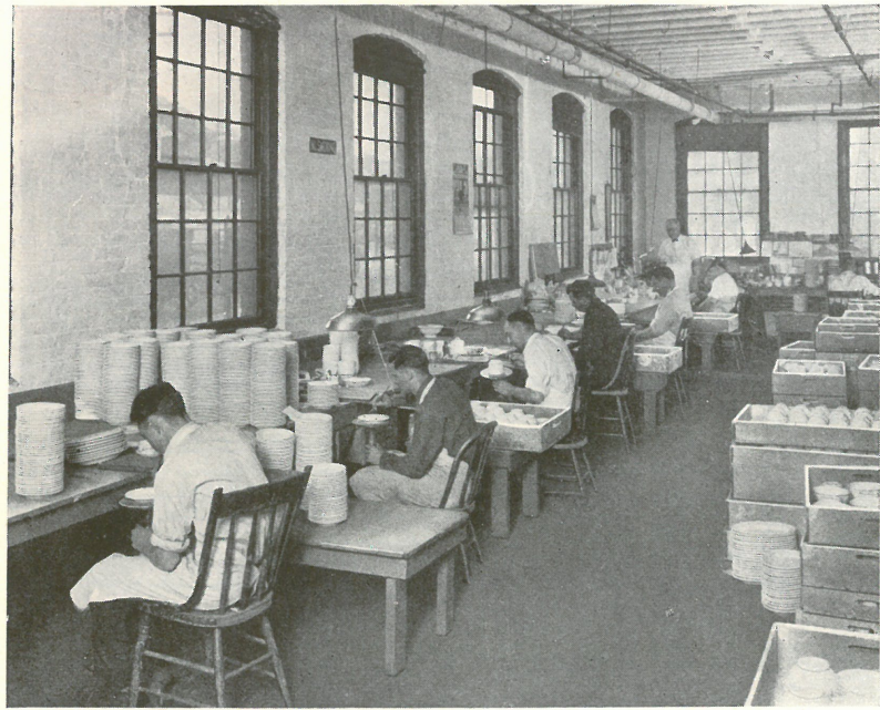
Band and line decorating room. Experienced decorators with dexterous brushes apply the color.
